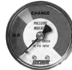
Y2—Back mounted 1/8" NPT Tri-color Glycerin-filled Gauge (0-60 psi) P/N LFT-134-2 Y2R—Same as Y2 but mounted on opposite side of standard location P/N LFT-134-2 Y2C—Bottom mounted 1/8" NPT Tri-color Gauge (0-60 psi) located in cap P/N LFT-134-3 Y5—Same as Y2 but located in cap P/N LFT-134-2 For 0-100 psi gauge, contact factory.
