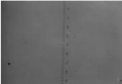
Figure 10. Microscopic Examination of an Oil Sample (100 ml) Magnification 100x (ISO 18/15/11)
